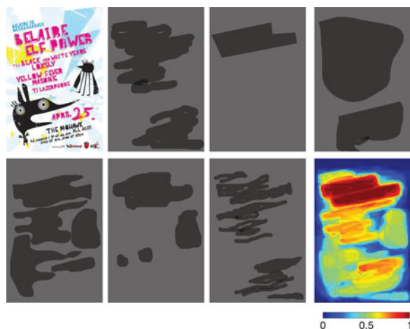
Fig. 2. Importance maps . Given a design (top left), MTurk users mark what they consider important. While the individual maps are noisy, when averaged over 20-30 users (bottom right), the mean maps are reasonable. Design courtesy of Flickr user Dániel Perlaky.
