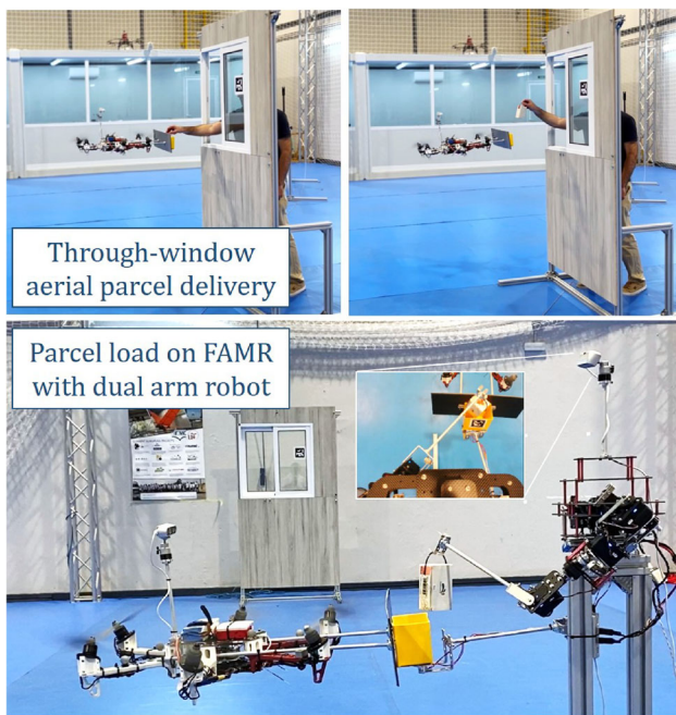
Fig. 1 Through-window aerial delivery system consisting of fully actuated multi-rotor (FAMR) and lightweight and compliant anthropomorphic dual arm system (LiCAS) located in the supply area used to load the parcel in the FAMR with the left arm while the right arm holds the basket base
