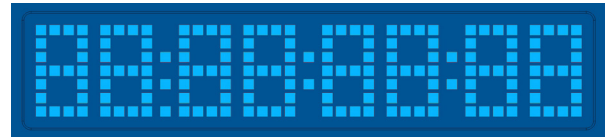
Blue - Timecode generator running
