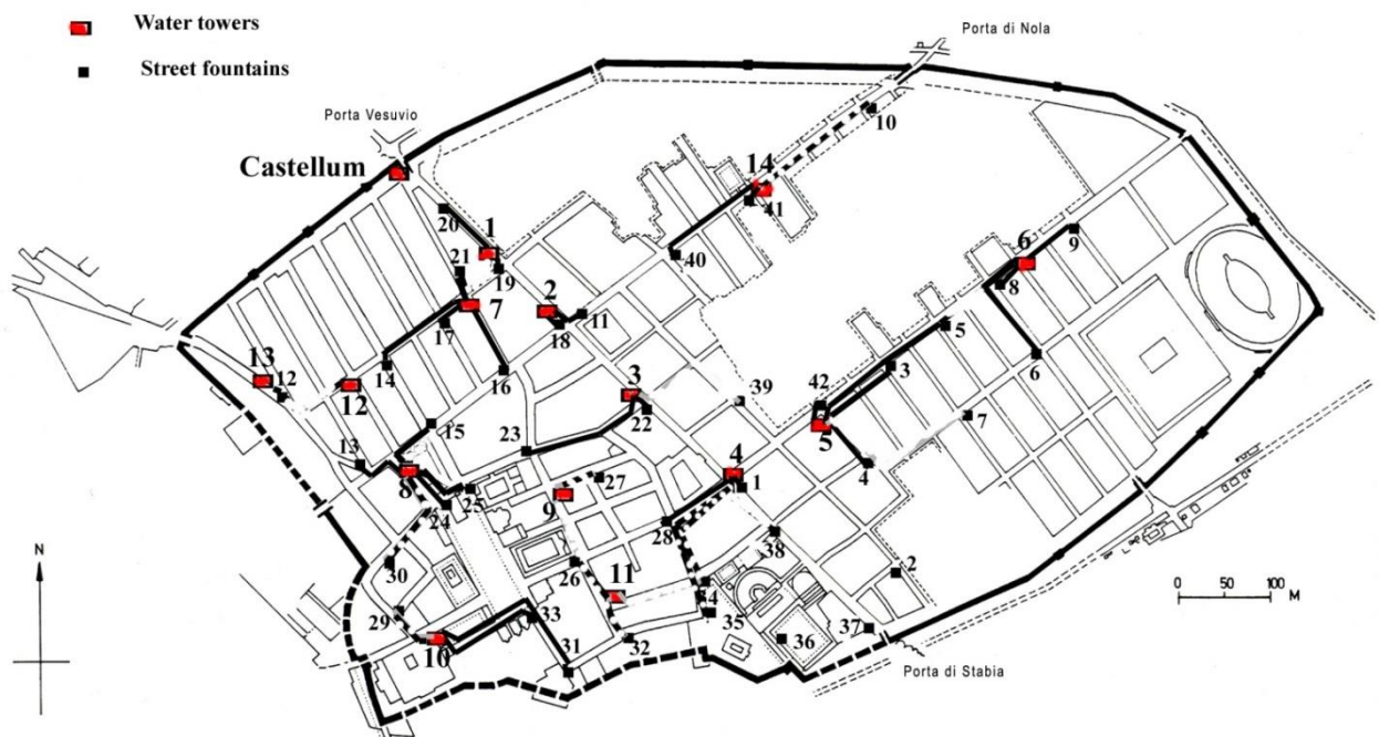
Figure 6.2. Plausible overall design of water-supply system to street fountains. Probable pipe connections to street fountains marked by solid lines and plausible connections, by dotted lines. Water towers in red. Drawing by author.
