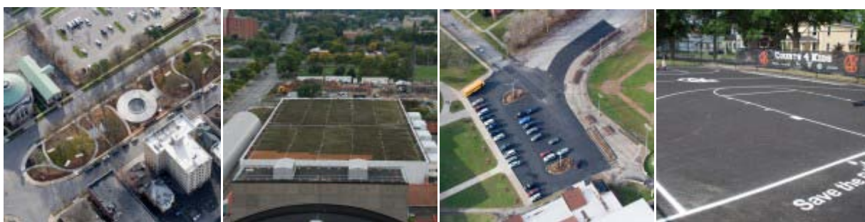
Figure ES-6 2011 Green Infrastructure projects part of the Project-50 program: (From Left to Right) Connective Corridor Forman Park, Green Roof at the OnCenter, porous parking lot for the Sunnycrest Arena, and Skiddy Park porous basketball courts.
