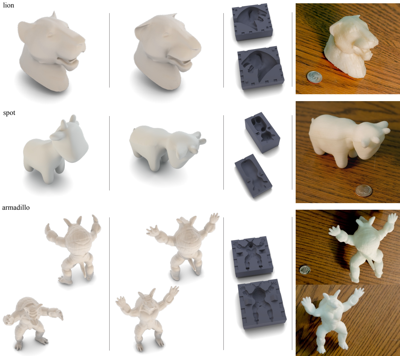
Fig. 17. Multiple casts fabricated via our method. The far-left column shows the input mesh; the left column shows the result mesh after applying our method; the right column shows the 3D-printed molds; the far right column shows the foam casts (dime for scale). The shapes undergo large deformations to become castable, but remain close to the input in terms of character.
