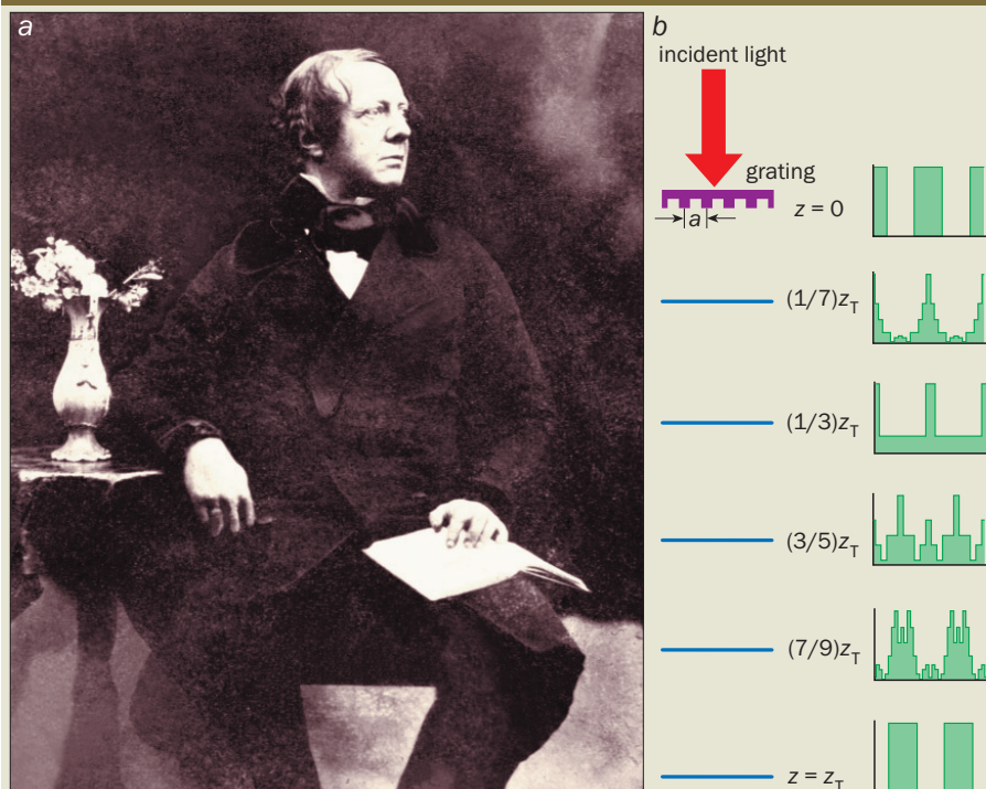
(a) Henry Fox Talbot (1800–1877) (Picture courtesy of The National Trust and the Fox Talbot Museum and kindly supplied by Michael Gray). (b) The Talbot effect from a Ronchi grating – a grating that has equally spaced transparent and opaque slits. The intensity pattern at the grating ( z = 0 ) is reconstructed at the Talbot distance z = z_T but is shifted by half a period. The images that can be viewed with the aid of a lens (not shown) occur at intermediate distances given by rational fractions p/q of z_T . These “fractional Talbot images” consist of q overlapping copies of the grating; several values of p/q are illustrated here. Neighbouring images are shifted by a/q , and coherently superposed with phases given by the Gauss sums of number theory (see box).
