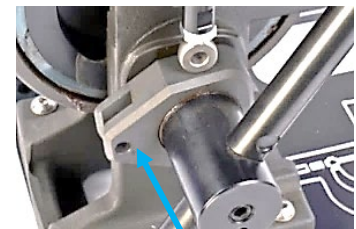
Rotate the Swage Con Rod Sideways to remove the Swage Rod--it may be necessary to remove the adjusting Eye Bolt (2) and Lock Nut (9) also
