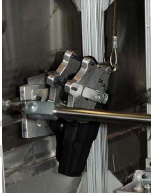
Example of Static Strength Fixture demonstrating the directions of loading and impact testing #1 (See Figure 1)
