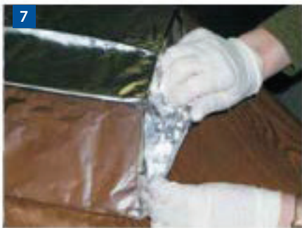
7 Roll the ends twice and press flat against the foam block.
