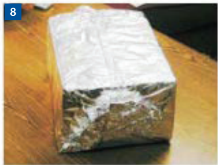
8 The finished foil wrapped sample should be tightly sealed on all sides. Remember: Only one sample per foil package.
