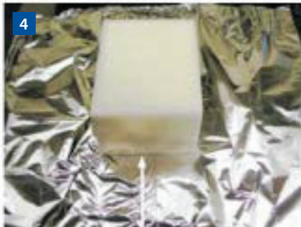
4 Place the foam sample in the center of the joined foil sheet lengthwise on top of the seam.
