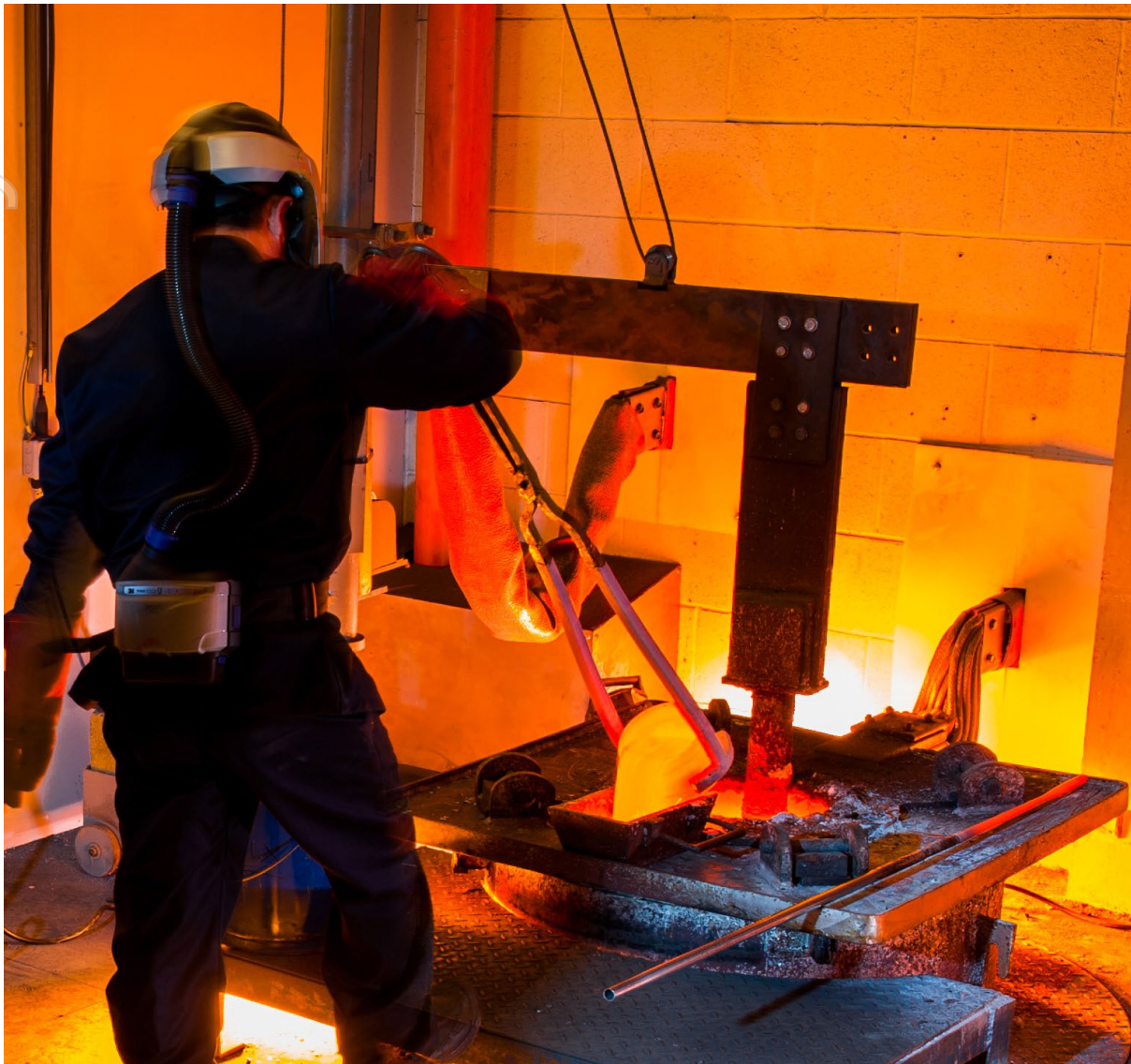
Figure 4: Rare earth metal alloy production via electrolysis at LCM (source: www.lesscommonmetals.com ).
