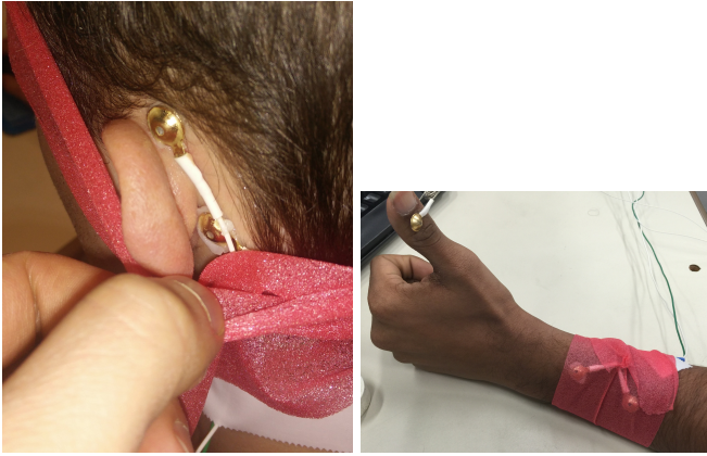
Fig. 2: For the user studies, the sEMG device was placed over the superior auricularis (SA) muscle, located behind the ear for 3 subjects, and over the extensor pollicis longus (EPL) muscles, located on the forearm for the other 3 subjects. The electrodes were attached with Ten20 conductive gel, and a small amount of prewrap (red) was used to stabilize them.
